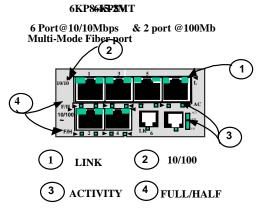
100Mb MTRJ fiber ports. When installed in a Magnum 6K16-Series Switch, it supports the standard distances as mentioned on 5.2.3. and the LEDs also act similarly.
